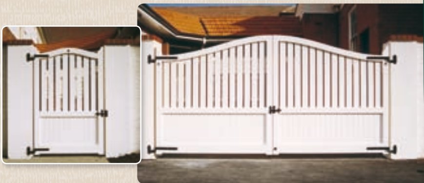
These Dempsey gates, leading into a private school, were chosen for solidity, security and elegance. They have been fitted with special hinges which allow them to be opened a full 180° against the wall. T/G&V at the bottom and ex 100x25mm palings with a 20mm gap at the top.
