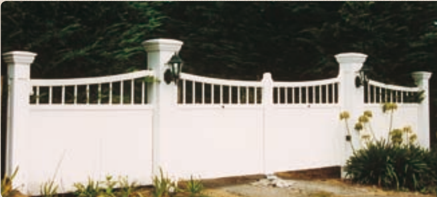
The Courtney's curved top rail gives an inviting atmosphere to the entranceway. T/G&V with 28mm dowels makes a very substantial gate, here hung on ex 300x300 feature posts with Replica Plain caps and with matching fence panels supported by ex 200x200 feature posts.
