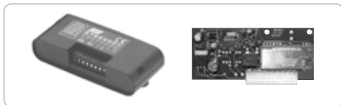
RX433/A super eterodyne and coupling code ACG5055 RX433/A super eterodyne and terminal board code ACG5056 RX433/A 2CH super eterodyne, 2 channel and coupling code ACG5051 RX433/A 2CH super eterodyne, 2 channel and terminal board code ACG5052
